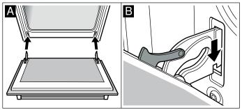
Fold back both locking levers (figure C). Close the oven door.
